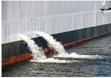
D-2 Commissioning Testing for BWTS
